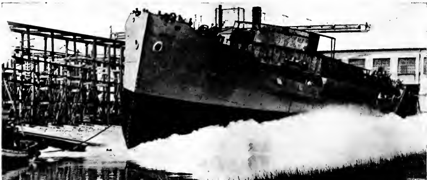
Side launching of one of the large number of small salt-water freighters building at the yards of the American Shipbuilding Company.
